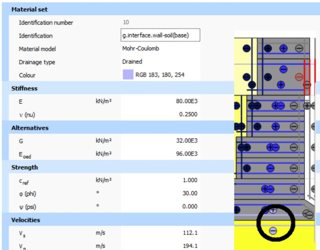
Figure 2.36: Interfaces at the base of the quay wall
