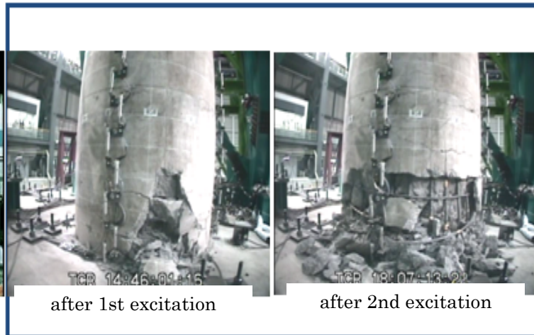
Photo1: Damage progress of C1-1 at SW surface
