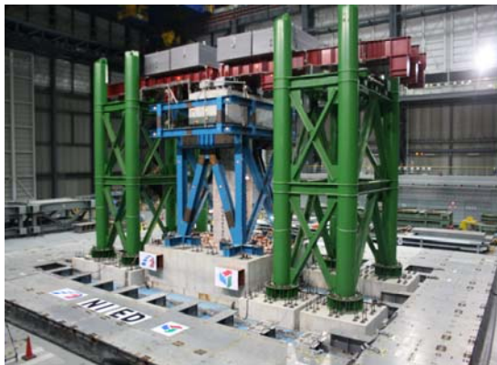
Photo3 : Experiment set-up on E-Defense shake table
