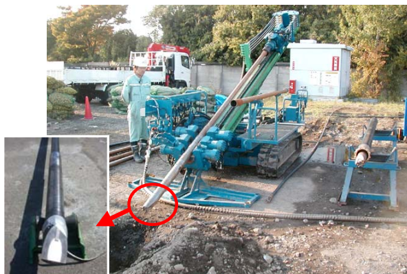
Figure 5. Drilling machine and the tip structure of rods
