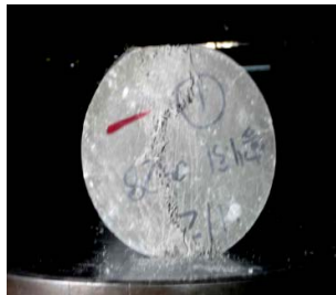
State of Test for splitting tensile strength
