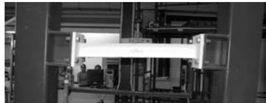
Figure 5. Testing of an IPE 100 as the connecting beam.
