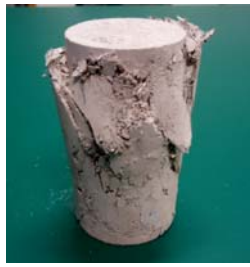
State of Test for Compressive strength of PFRC
