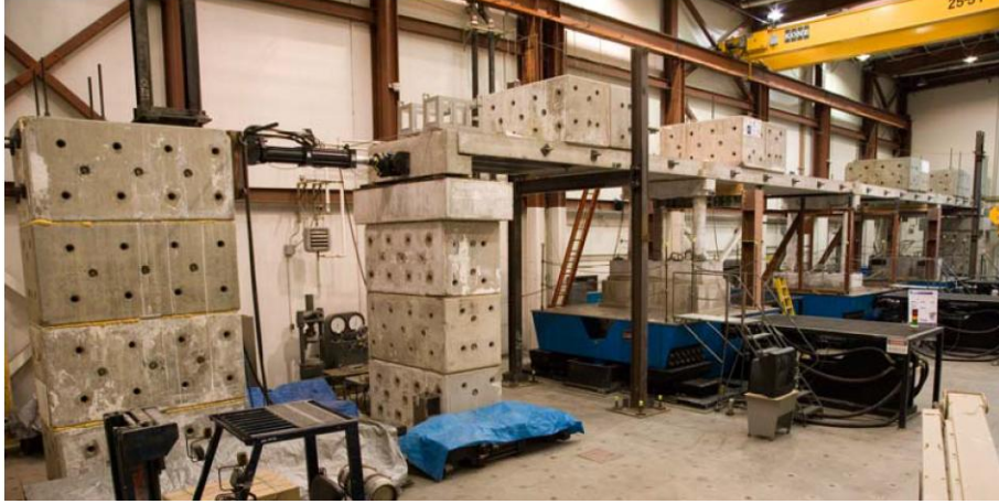
Figure 8. Quarter-scale bridge model on shake Tables
