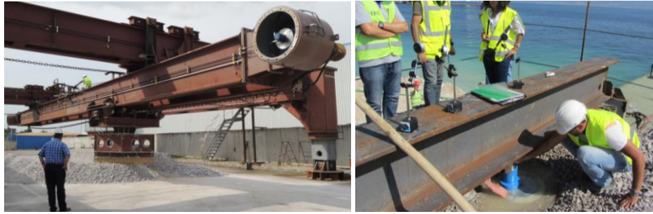
Figure 13. (a) Demonstration of sub-sea levelling unit; (b) Plate loading test on “retrieved” gravel
