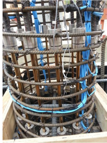
Figure 3. Reinforcing SMA bars used in plastic hinge
