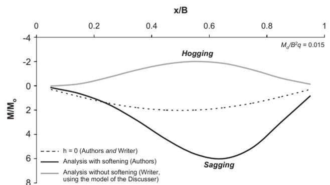
**Fig. 7.** Analysis of rigid  $B=10$  m foundation with superstructure load  $q=20$  kPa, subjected to  $h=2$  m normal faulting ( $\alpha=60^\circ$ ) through idealized dense sand, at  $s=1$  m
