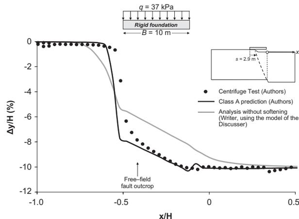
Fig. 4. Test 15: rigid  $B=10$  m foundation with superstructure load  $q = 37$  kPa, at  $s=2.9$  m
