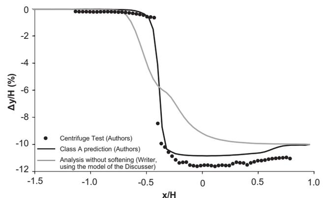
Fig. 2. Test 12: normal faulting at 60°, soil with  $D_r=60\%$
