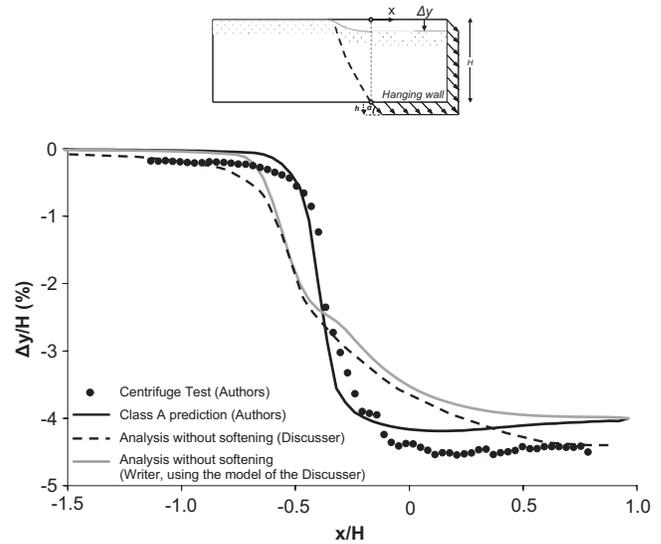
Fig. 1. Test 12: normal faulting at 60°, soil with  $D_r=60\%$
