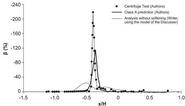
Fig. 3. Test 12: normal faulting at  $60^\circ$ , soil with  $Dr=60\%$
