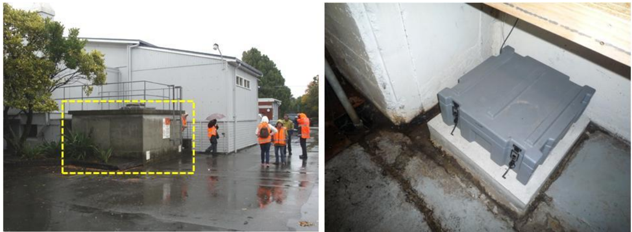
Figure 2.9. The basement accommodating the seismic station (left) and the seismograph placed in a box fixed on the solid base on the ground floor (right).
