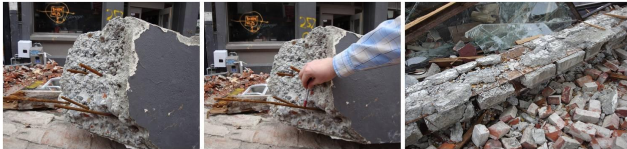
Figure 3. 15. Insufficient reinforcement, low quality concrete and bad application caused collapse of a decorative beam and 1 casualty.
