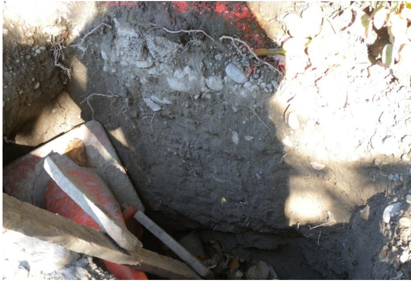
Figure 2.36. Excavation near the CBGS seismic station showing part of the superficial soil deposit consisting of silty sand.
