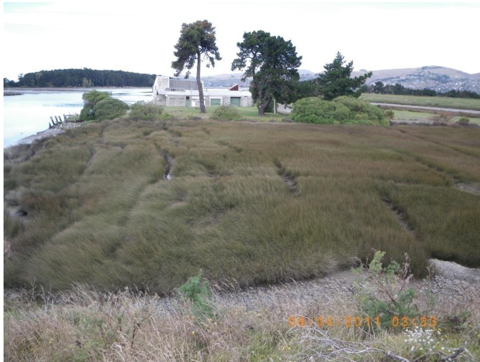
Figure 5.32. South Bridge Road Bridge (B8 on map of Figure 5.1) after Christchurch earthquake. Large lateral spreading cracks in the ground parallel to the coast and adjacent to the abutments extending at a great distance inland.
